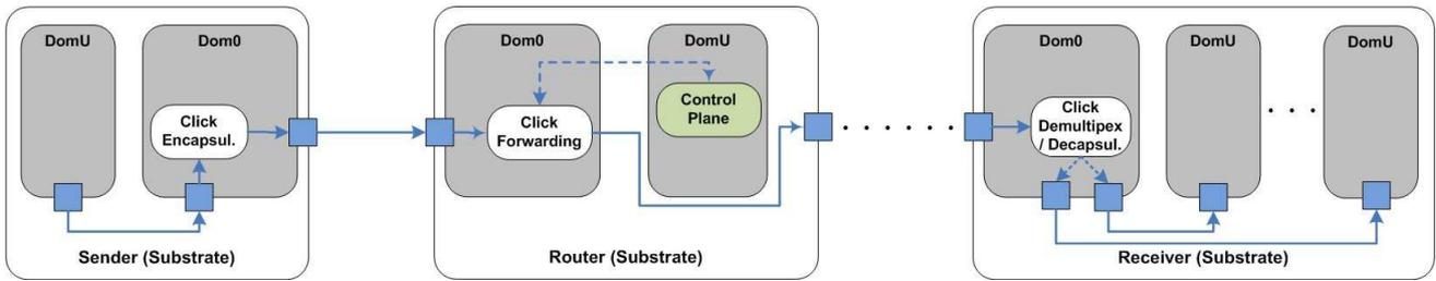
Fig. 5. Virtual Links on the Prototype
