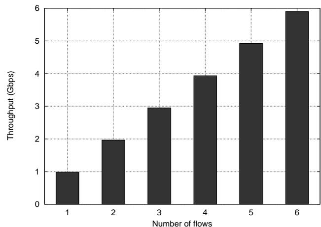
Fig. 8. Throughput with 1500-byte packets.
