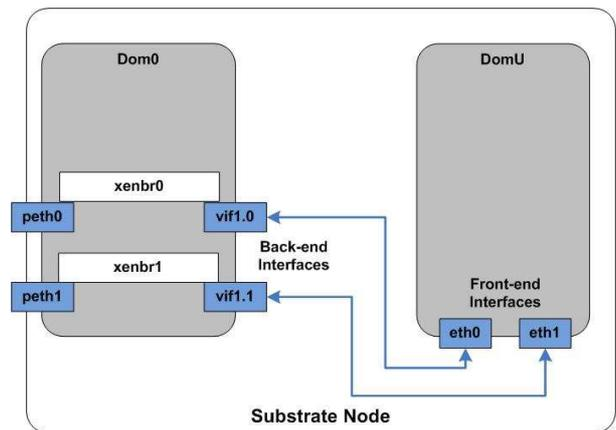
Fig. 4. Substrate Node with Bridged Configuration
