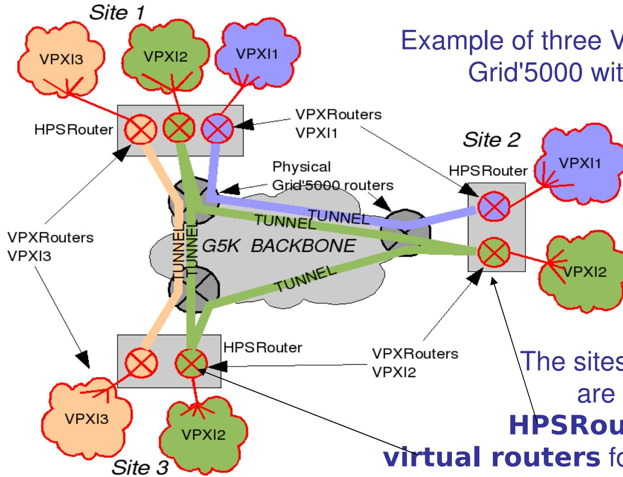
Example of three VPXIs allocated on Grid'5000 with HiperNET
